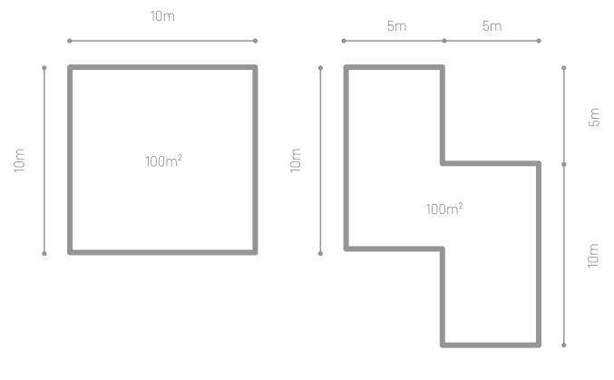
Figure 2: Structures with equivalent surface areas and different perimeters
