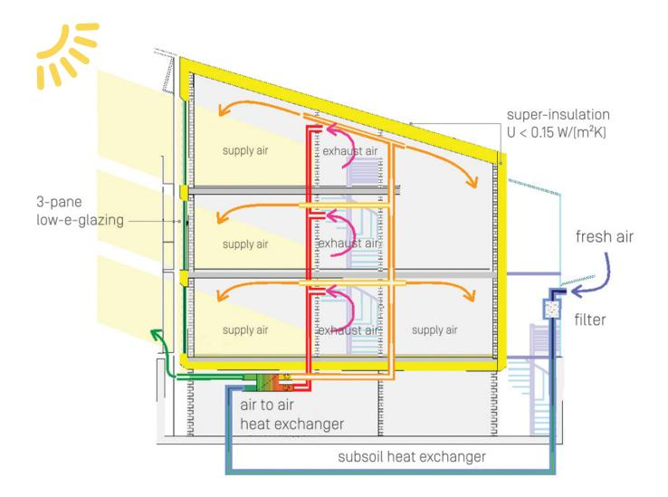
Figure 1: Cross section of a typical Passivhaus structure <sup>11</sup>
