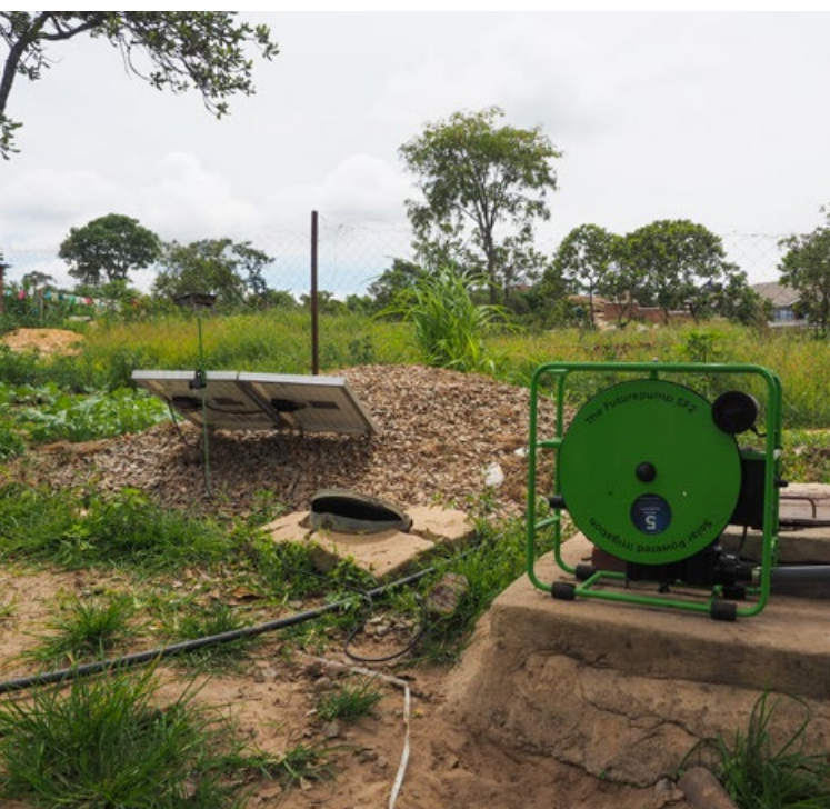
Celfre Energy is a locally-owned company distributing robust and portable solar water pumps in Zimbabwe. Each unit can pump one litre of water per second.
