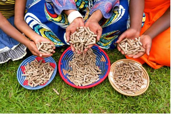
The biomass pellets are a long lasting and efficient fuel source, requiring about 90% less wood for production as compare to charcoal. No smoke is generated through the cooking process and the GHG and toxic emissions are reduced by 98%.
