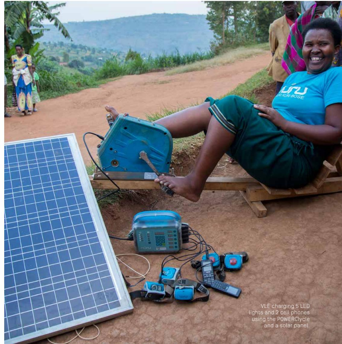
VLE charging 5 LED lights and 2 cell phones using the POWERCycle and a solar panel.
